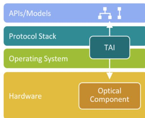
As part of this project, we integrated open-source TAI library in to NOS and developed TAI complaint vendor specific driver modules, the architecture of which is as shown below.
