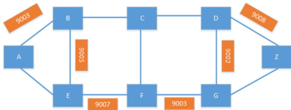
It is also possible to combine the node SID and adjacency SID to create a custom traffic policy. Labels are specified in a label stack, which may include several labels. By combining labels, you can create policies such as, "Send the traffic to F; I don't care how you get there. From F, go to G, then to D and then finally to Z." This creates endless possibilities for traffic engineering in the provider network.
